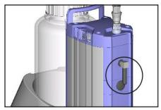
Removing the connection tubing from the screw cap leads to immediate venting of the
