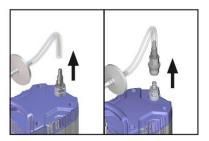
Remove screw cap from the collection bottle after venting.
