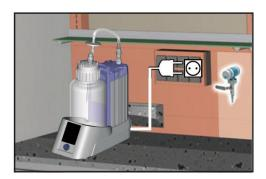
3. Attach tubing to the hose nozzle of the bottle head
