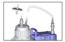
Attach new filter. Observe flow direction. Position filter with the printed side "IN" towards the bottle. Attach the connecting tube.
